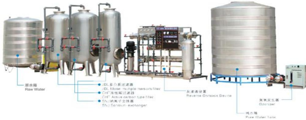
Raw water→ Raw water tank→ Multistage centrifugal stainless pump→ Multi-medium filter →Active carbon filter→sodium-exchanger→ Micro filter→Reverse osmosis → UV sterilizer →Pure water tank →Pump
